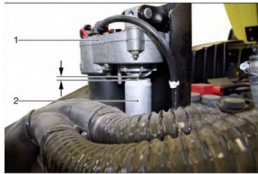
1 Lifting motor 2 Spindles
